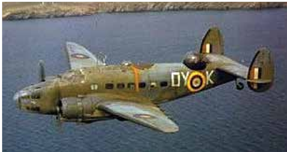
During the war, many Hudsons were fitted with both a turret (toward the back of the fuselage) and an astrodome (further forward), where Jack Dods spent much time while in flight.
